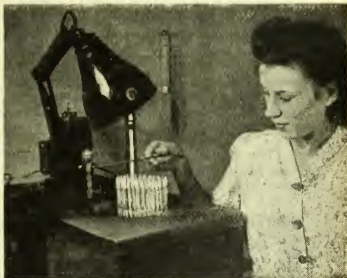
Removing thermometers from calibration bath. Below: Dividing the scale on wax-covered thermometer
